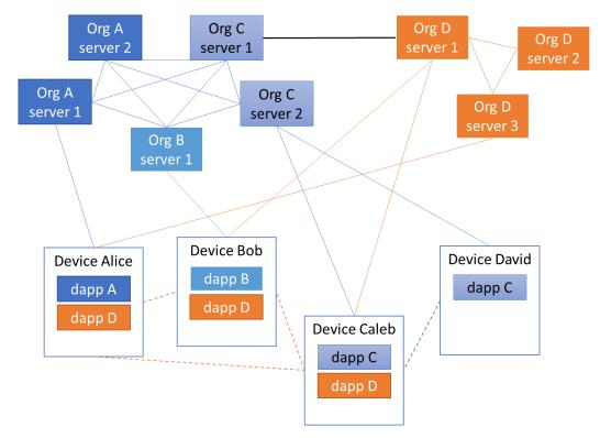
This diagram shows a network of 8 servers and 4 devices. Organizations A, B and C are running a permissioned blockchain that handle transaction and store states of 3 dApps : dapp A, dapp B and dapp
